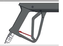
Disconnect the CO<sub>2</sub> hose from the CO<sub>2</sub> quick connector on the gun.
