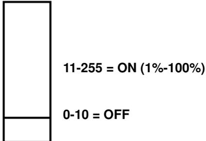
**If the value of channel A is set between 0 to 10, the unit is off.**
