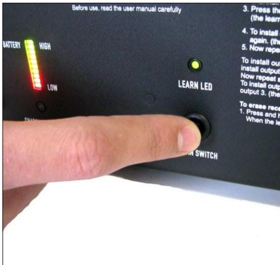
To make the Shot Base Wireless react to a remote 4/8 turn on the remote and press the LEARN SWITCH on the Shot Base Wireless, now the LEARN LED will blink once. This means output 1 can be programmed to button on the remote.
