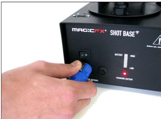
If u want to use the Shot Base Wireless on a location without an constant power supply u need to charge the Shot Base Wireless first.
