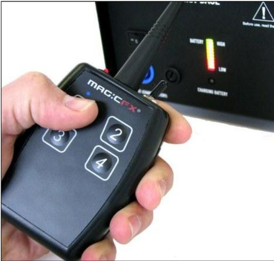
Press the button on the remote u want to assign to output 1. The LEARN LED on the Shot Base Wireless will light up. Press the same button on the remote again to confirm your setting. The LEARN LED will blink to confirm your setting.
