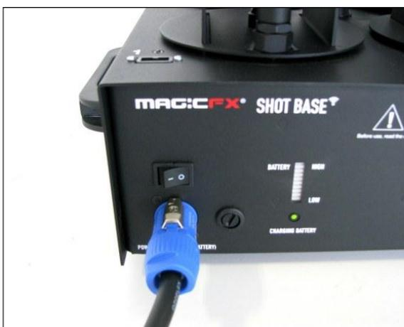
When the Shot Base Wireless is fully charged (the LED CHARGING BATTERY is green) u can choose to unplug the Shot Base Wireless and use it wireless
